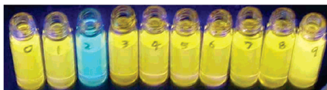
FIGURE 4. Fluorescence response of RMS in the presence of 20 equiv of different metal ions. Conditions: 10 \mu M RMS in 0.05 M HEPES 13 -buffered water solution (pH = 7.5). 0, control. 1, Cd 2+ . 2, Hg 2+ . 3, Fe 3+ . 4, Zn 2+ . 5, Ag + . 6, Co 2+ . 7, Cu 2+ . 8, Ni 2+ . 9, Pb 2+ . The salts employed are Cd(NO 3 ) 2 ·4H 2 O, HgCl 2 , Fe(NO 3 ) 3 , Zn(NO 3 ) 2 , AgClO 4 ·H 2 O, CoCl 2 ·6H 2 O, Cu(ClO 4 ) 2 ·6H 2 O, NiCl 2 ·6H 2 O, and Pb(ClO 4 ) 2 ·3H 2 O, respectively.
